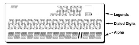
Figure 13 - Phonecell SX4D LCD Display.
